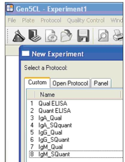
Gen5CL allows the user to select a pre-programmed protocol from the installed assay database, or to create their own protocols from the open protocol interface.
