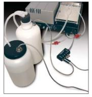
The Liquid Level Alert<sup>™</sup> option allows users the convenience of continuous monitoring for both supply and waste bottles. At the beginning and end of a wash protocol, the liquid level is verified to ensure sufficient wash buffer remains in the designated dispense bottle to complete a microplate wash. Sufficient storage capacity in the waste bottle is also verified.
