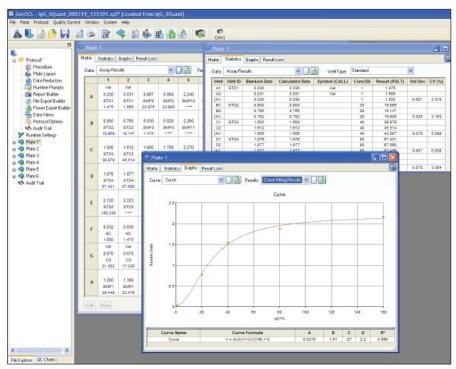
Gen5CL's data views can be customized to show preferred data sets from one plate or multiple plates in an experiment.
