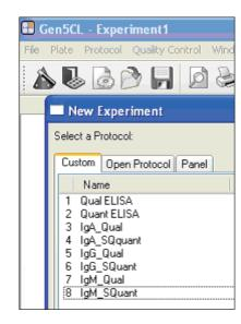
Gen5CL allows the user to select a pre-programmed protocol from the installed assay database, or to create their own protocols from the open protocol interface.
